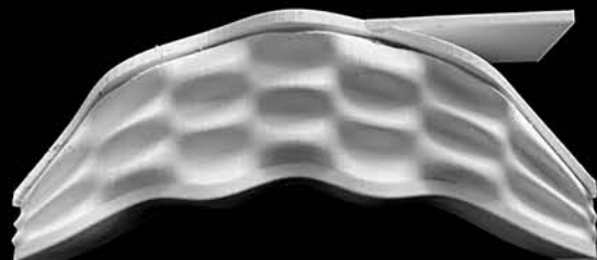
Silicon casting on a 3d printed mold
